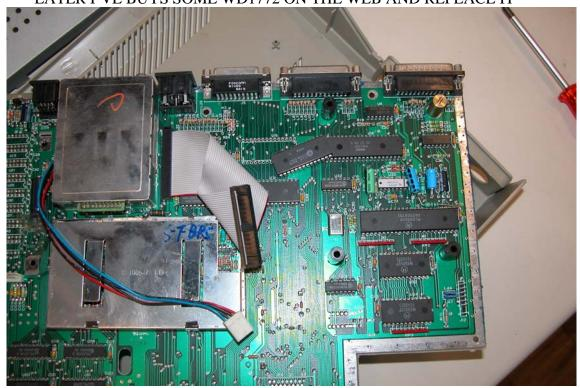
After soldering the dual in line FDD connector I've insert the plastic for the FDD Connector. You can see the location of a missing 1kohm pull-up resistor pack "RM5". You must solder this resistor pack or 5 x 1khm resistors with the common at the right side of the picture (opposite to the "RM5" indication)
