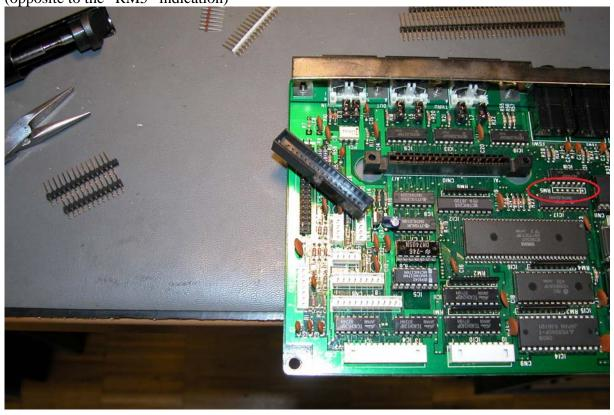
I've insert and solder 5 IC sockets, remove the Battery and insert the Battery socket removed from the PC Main Board.
