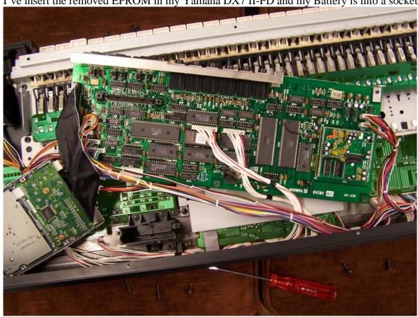
I must make a hole for the Floppy and a little mechanic and a good Power Cable for FDD
