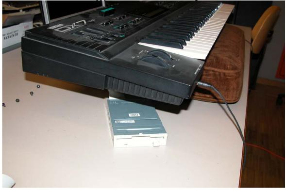
New Floppy Disk mounts. I must still make a short flat cable and a good FDD Power Cable.
